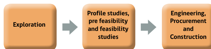
Figure 1.1 - Stages of a Mining Project prior to Operation
